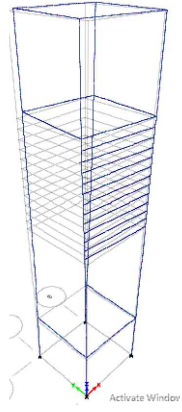
Figure: Deformed Shape due to Wind x
