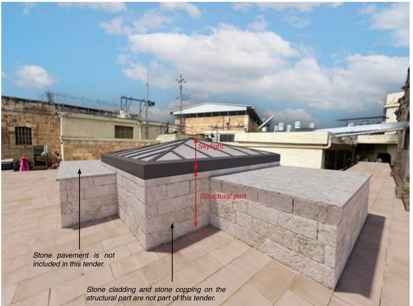
3D image of the Room C skylight, view from the roof - P&R
