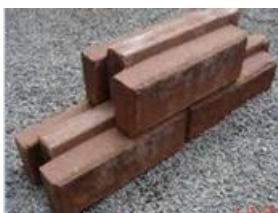
Picture: showing male, female interlocking features, grooves and smooth intact edges plus surfaces
